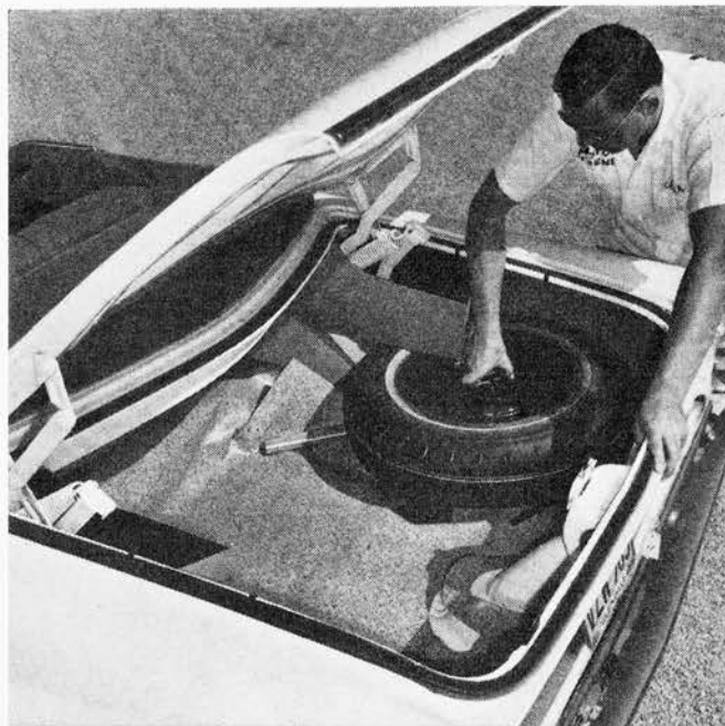
Trunk is wide and long but not deep. It still provides a lot of room for the easy-to-reach spare plus an average load of luggage. Cardboard shield defines the hinge area.
