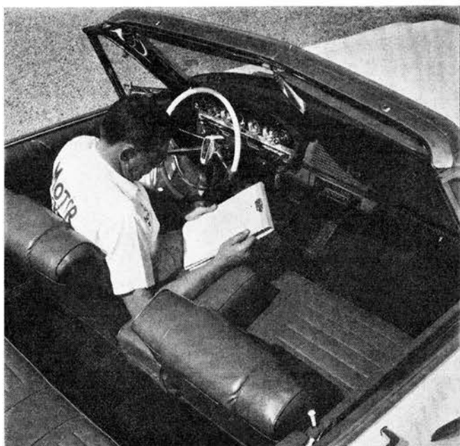
The split-back front seats are comfortable and offer good support to the back and thighs. The fore-and-aft adjustment is adequate. The pull-down armrest comes in handy.
